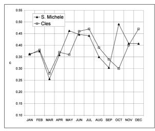
Fig. 2 - Values of the coefficient "c" for the assessment of sunset temperature - see equation 5 - calibrated monthly over a 27-year period (1983 - 2009), stations of S. Michele and Cles.
