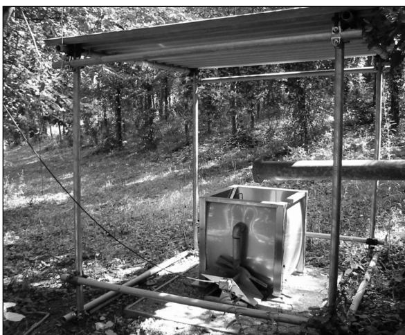
Fig. 3 - Experimental station for the measurement of runoff and the collection of samples.
