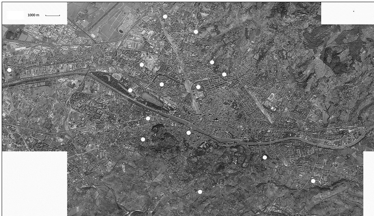
Fig. 1 - Florence Municipality map and location of the 15 air temperature and relative humidity sensors.
